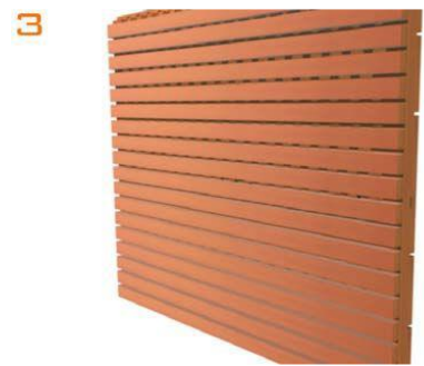
2 Install subsequent tongue and grooved panels and secure with Fixing Clips
